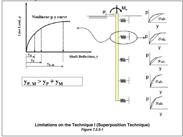
Designers should be careful to match the geometry of the FEM and soil response program. If the location of the foundation springs (or node) in the FEM does not match the location input to the soil response program, the two programs will not converge correctly.
