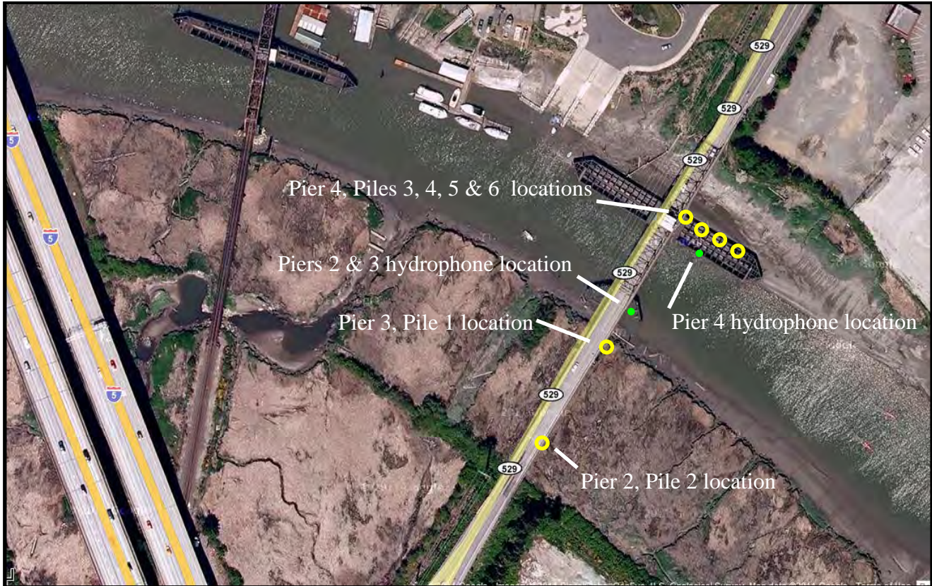
Figure 2: Approximate location of 72-inch piles and hydrophones at the SR 529 Ebey Slough Bridge Replacement Project.
