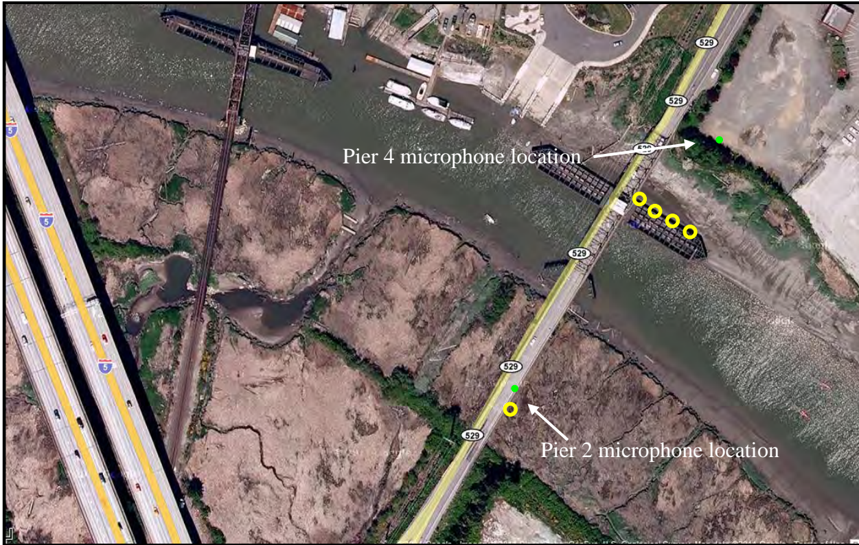
Figure 20: Location of airborne noise measurements at the SR 529 Ebey Slough Bridge Project. ○ = 72-inch Steel Pile; ● = Airborne Microphone
