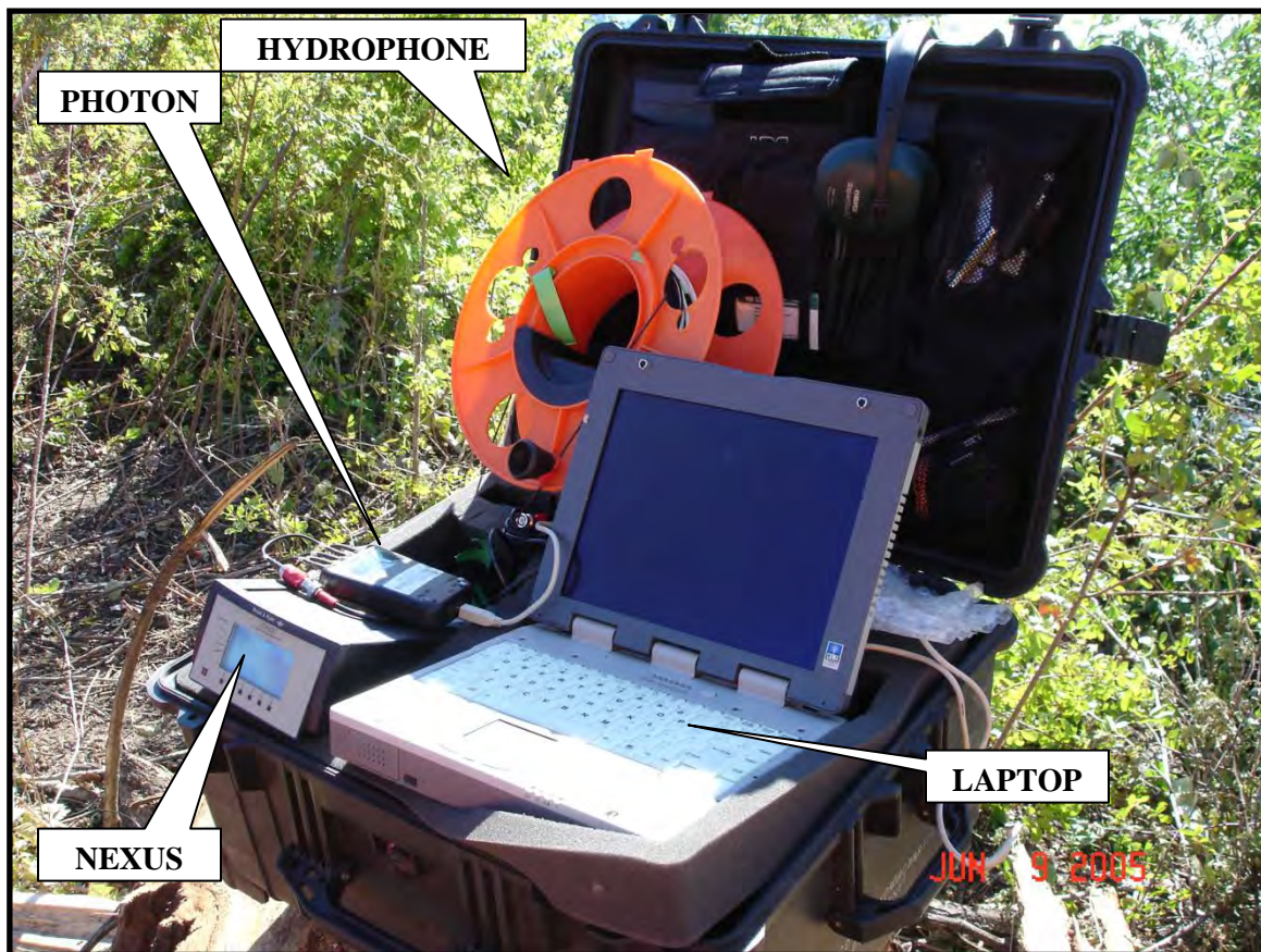
Figure 3: Near field acoustical monitoring equipment
